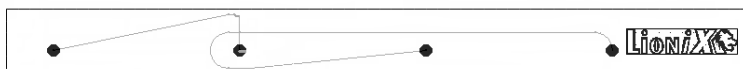
Fig. 3.2 Layout of the MF chip - design 2, with a much shorter sample injection channel (reservoir 1 \rightarrow reservoir 2) with less kinks, incorporating MF channels with cross-section dimensions of 110\ \mu\text{m} \times 50\ \mu\text{m} , breadth \times height.
