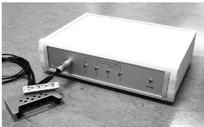
Fig. 3.5 Picture of the capilix system for flow control in the optofluidic chip
